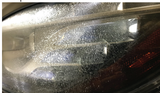
Example of nonrepairable crazing damage
